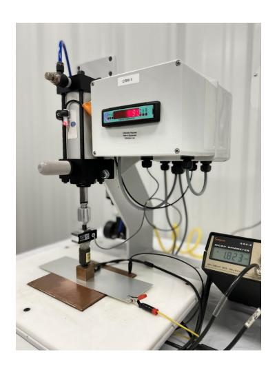
In-House Contact Resistance Testing for Chromated Aluminum Metal Finishers
